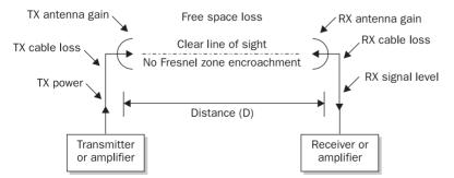
Figure 17-3 Wireless link power gain and loss
