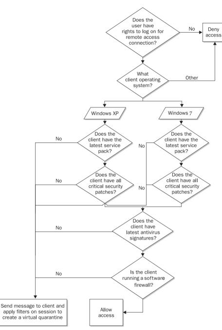
Figure 16-4 Sample quarantine logic for the authentication of end-user computers to VPN
