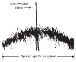
**Figure 17-5** Spread spectrum versus narrowband transmission
