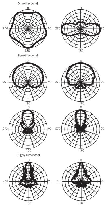
**Figure 17-1** Examples of antenna irradiation patterns supplied with quick antenna type-specific beam-width reference values
