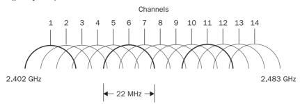
In Europe, 13 channels are allocated for 802.11b/g use, making access point coallocation more flexible (however, only the channels from 10 to 13 are used in France and 10 to 11 in Spain). All 14 channels can be used in Japan. Channel allocation has high relevance to the much-discussed issue of *rogue access points*. There are various definitions for a "rogue access point" and, therefore, different ways of dealing with the problem:
