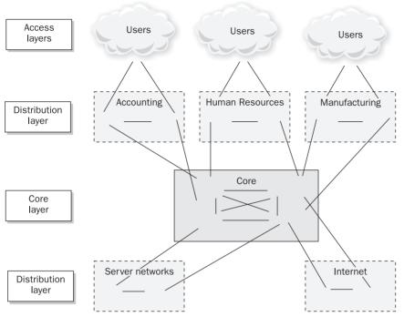
Figure 13-1 The Cisco Hierarchical Internetworking model
