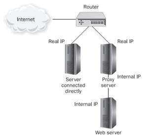
Figure 23-8 A reverse proxy configuration
