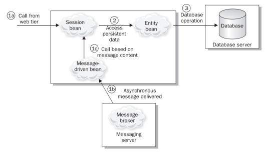
Figure 28-3 Typical EJB configuration
