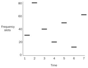
Figure 17-6 FHSS frequency hopping
