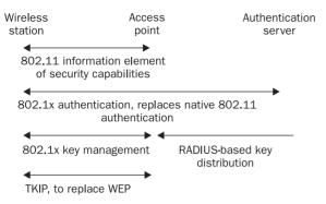
Figure 17-12 An overview of 802.1x/TKIP functionality
