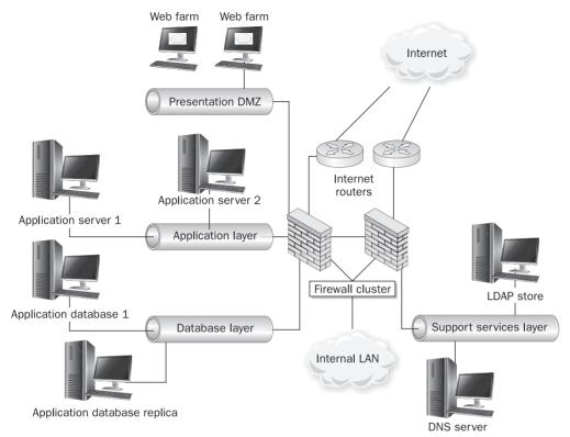
Figure 13-7 Example of a multitier application infrastructure
