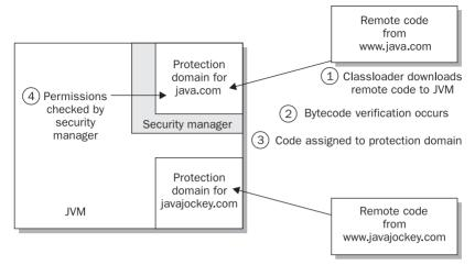
Figure 28-1 A JVM partitioned with a security manager and protection domains
