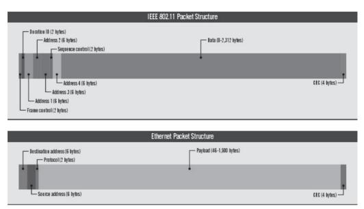
Figure 17-8 Comparison between 802.11 and 802.3 frames
