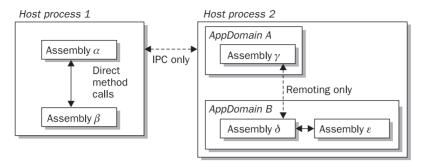
Figure 29-7 Use of AppDomains for assembly isolation
