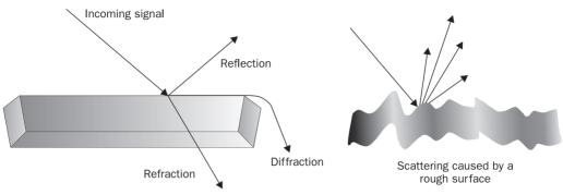
Figure 17-4 Electromagnetic wave-object interactions
