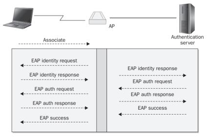
Figure 17-13 EAP authentication process
