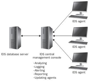
Figure 18-2 Example of a distributed IDS topology
