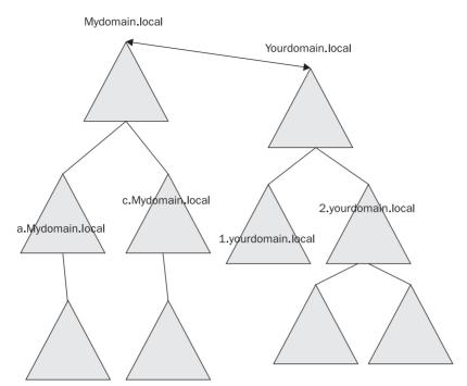
Figure 22-7 Kerberos-style two-way transitive trust between two forests
