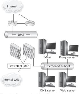
Figure 13-6 A sample DMZ configuration
